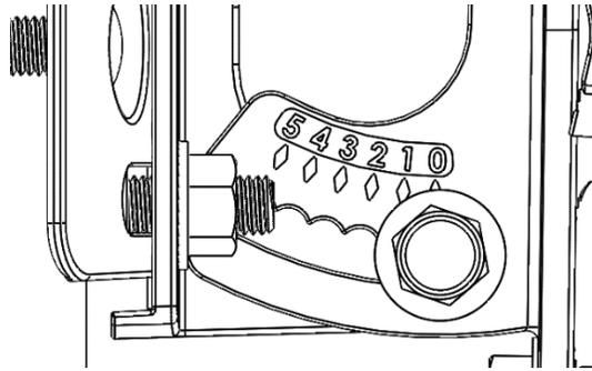
9. The CPE can be adjusted by sliding the mid bracket left and right after loosening the lock nuts installed in Step 2 (above). There are scorings every 7° of azimuth-angle from 0 (0° position) to ±2 (14° position left or right). Tighten the lock nuts when satisfied with the position of the CPE.
