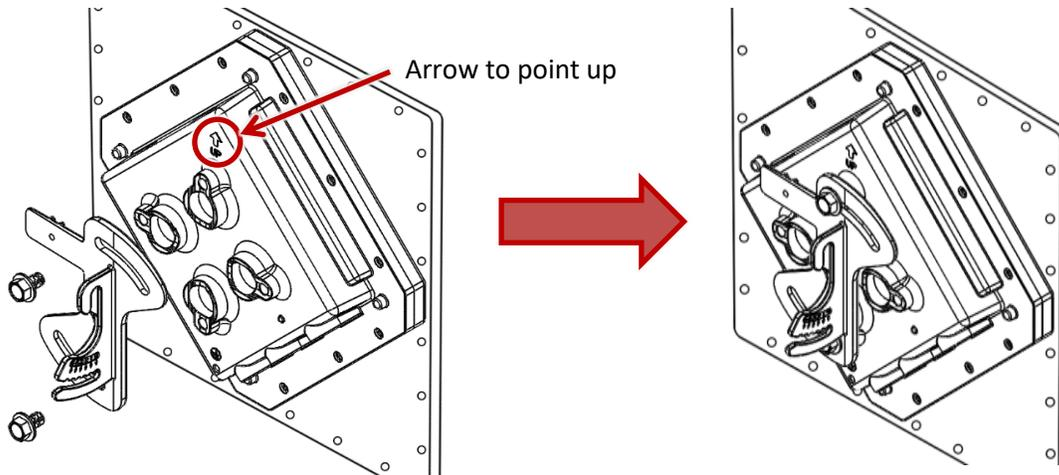
7. Bring the CPE up to the previously secured bracket on the pole. Hook the unit side bracket (there is a small hook on the top) onto the loosely fastened M10x1.5 screw on the mid bracket – such that the hook is on the screw itself. Tighten the screw to secure the unit.
