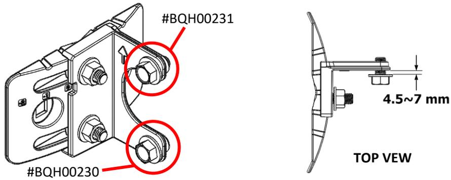
4. SECURING BRACKET ON POLE: Take the assembled pole side bracket, hold it on one side of the pole. Slot the two M10 carriage bolts (#BQH00228) through the holes of the bracket and hold it there; take the clamp (#BQF00308) and slot it through the carriage bolts. Fasten the bolts with two M10x1.5 lock nuts (#BQH00232).
