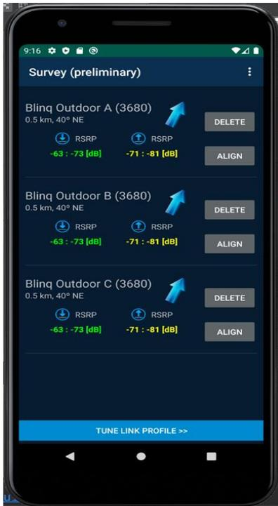
8. The **Alignment** CPE screen on the app to show the direction that the CPE is aiming (in **GREEN**) and target eNB direction (the **BLUE** arrow points to the eNB)
