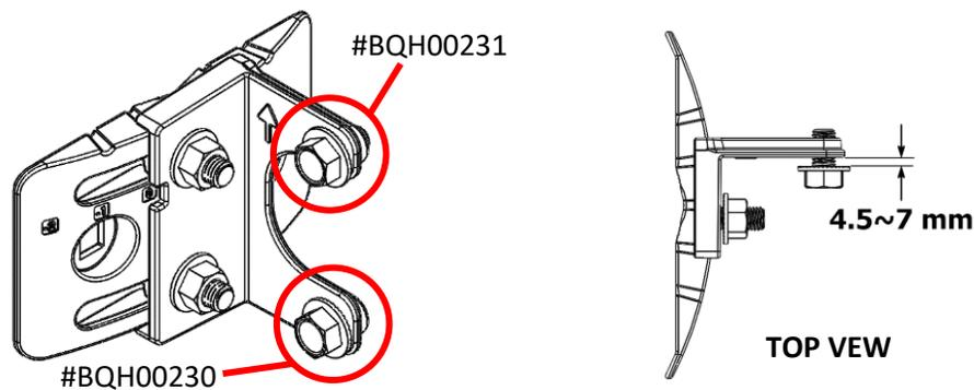
4. **SECURING BRACKET ON POLE:** Take the assembled pole side bracket, hold it on one side of the pole. Slot the two M10 carriage bolts (#BQH228) through the holes of the bracket and hold it there; take the clamp (#BQF00308) and slot it through the carriage bolts. Fasten the bolts with two M10x1.5 lock nuts (#BQH00232).
