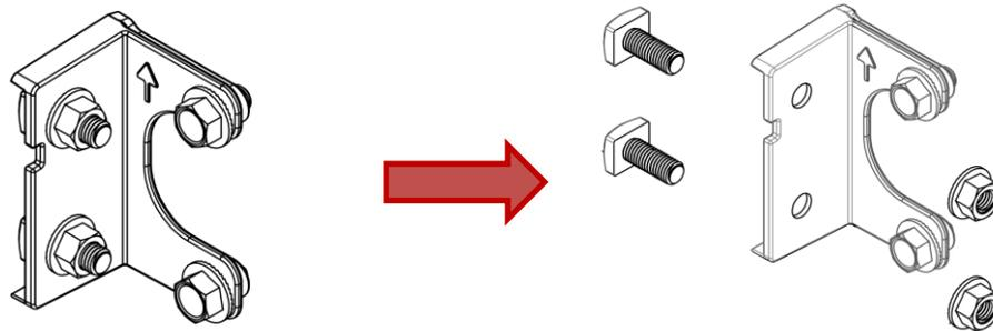
2. Secure the pole side bracket (#BQF00309) with the mid bracket by inserting two M10x1.5 (25mm L) screws through both brackets and fastened with two M10x1.5 lock nuts. Please take note of the mid bracket's orientation, ensuring that the arrow is pointing up. Position the mid bracket in the middle position of pole side bracket and adjust it after attaching the CPE (See Step 9)
