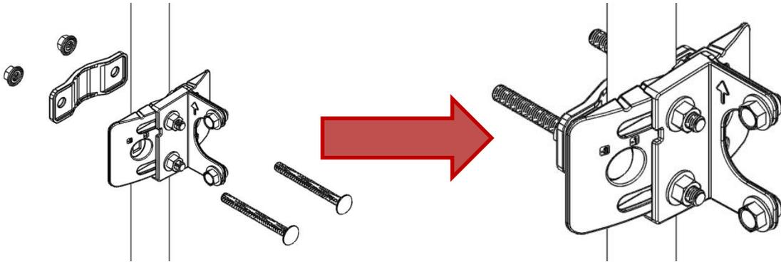
5. To assemble the unit side bracket, take the CPE and ensure that it is oriented with the arrow pointing upwards. (see figure below)
