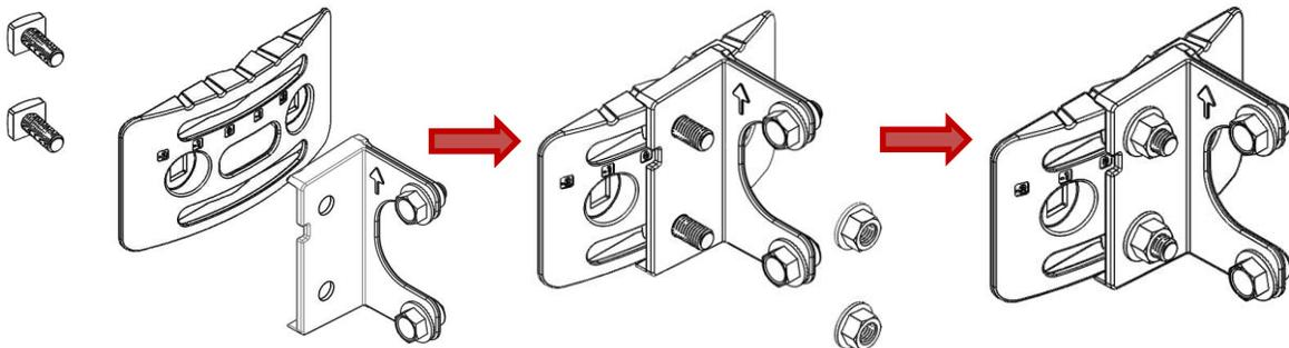
3. Please ensure that the M10x1.5, 16mm L screw (#BQH00231) on the top hole and the M6 enlarged hex head screw (#BQH00230) on the bottom hole of the mid bracket have a distance of 4.5-7mm between the screw heads and the mid bracket surface as shown in the top view figure below.
