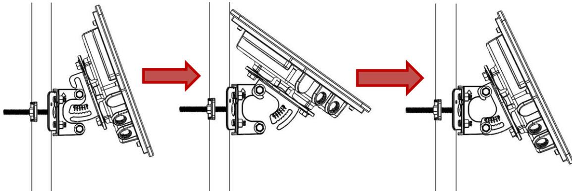
8. Then, slide the curved bottom part of the bracket onto the M6 enlarged hex head screw. There are scorings every 5 degrees of tilt-angle, from 0 (Vertical position) to 5 (25° uptilt). Adjust the tilt to the desired angle and tighten the screw to secure the position of the CPE.
