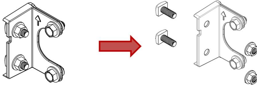
2. Secure the pole side bracket (#BQF00309) with the mid bracket by inserting two M10x1.5 (25mm L) screws through both brackets and fastened with two M10x1.5 lock nuts. Please take note of the mid bracket's orientation, ensuring that the arrow is pointing up. Position the mid bracket in the middle position of pole side bracket and adjust it only after attaching the CPE (See Step 9).
